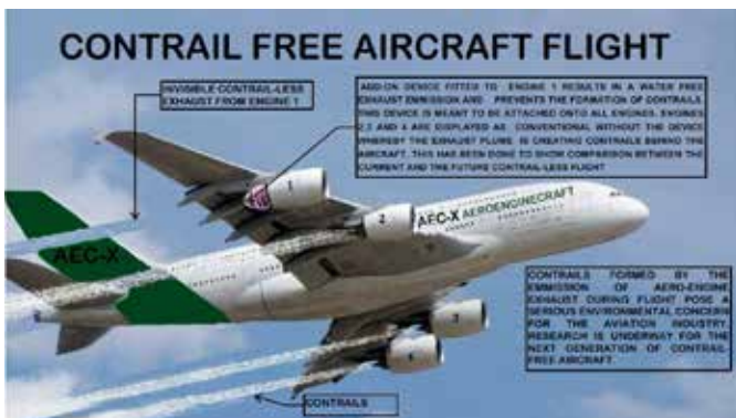
Figure 2: The concept behind a green contrail-free aero-engine
