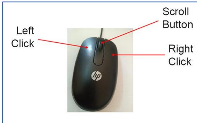
Figure 21: A typical mouse and its buttons
