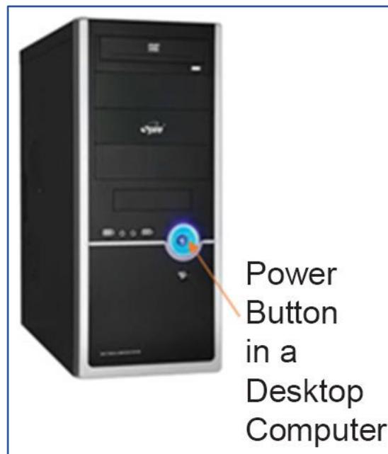
Figure 13: Typical location of a power button on a desktop PC
